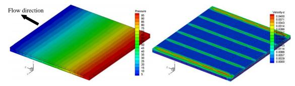
Fig. 4 Flow along the  $0^0$  direction of the big unit cell: (A) pressure contours; (B) velocity contours.
