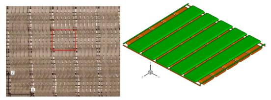
Fig. 1 (A) A photo of the biaxial fiber mat. (B) The big unit cell showing the two fiber-tow directions.
