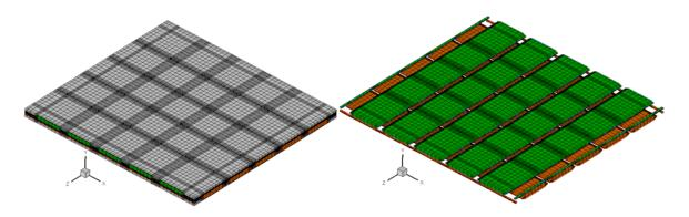
Fig. 2 Finite element mesh for the big (true) unit cell: (A) the whole unit cell; (B) just the fiber tows.
