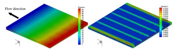
Fig. 5 Flow along the 90<sup>0</sup> direction of the big unit cell: (A) pressure contours; (B) velocity contours.
