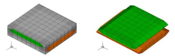
Fig. 3 Finite element mesh for the small (apparent) unit cell: (A) the whole unit cell; (B) just the fiber tows.
